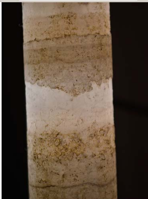
A core sample from the Borgen Bed from WMU's Geological Repository for Research and Education. The bed is a deposit of high-quality potash, a mineral used for fertilizer.
